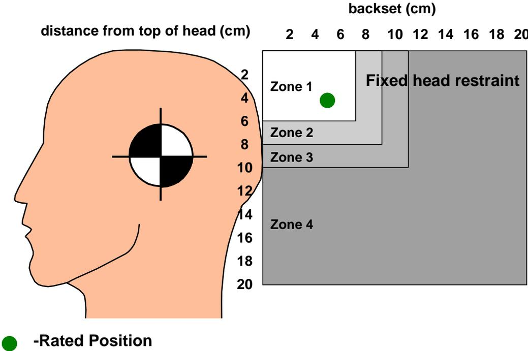
HEAD RESTRAINT RATING (HEIGHT ADJUSTMENT) NON LOCKING
