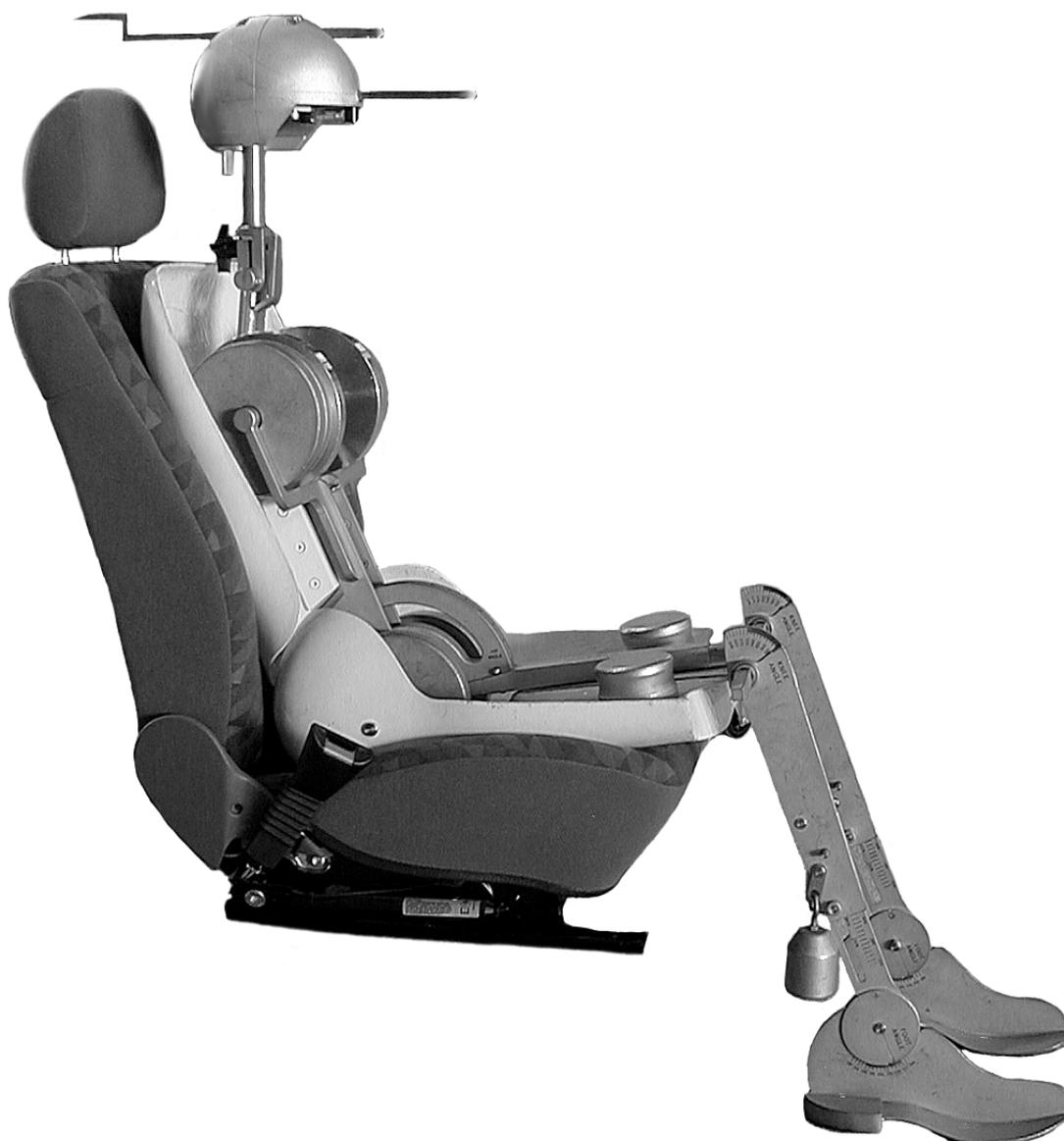
**Head Restraint Height Measurement**
